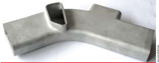
This hydroformed connecting node for an A-Pillar illustrates the high formability of stainless steels. (The original tube was rounded and straight.)
