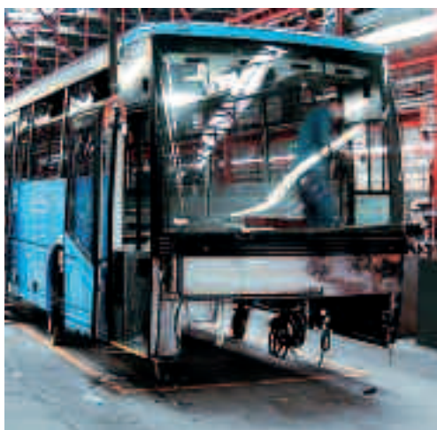
Figure 25: Used for buses and coaches, stainless steel (usually a painted ferritic grade) has proved compatible with a carbon steel chassis.
