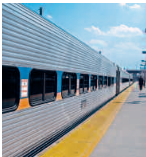
Figure 26: Rail coaches with outer panels in austenitic stainless steel have been used in many parts of the world, without galvanic corrosion problems.
