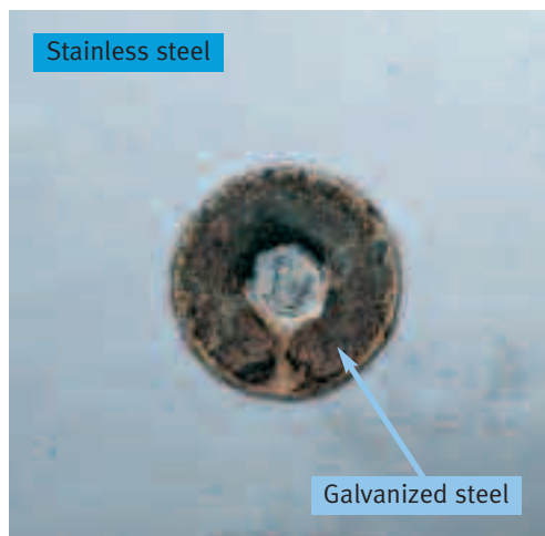
Figure 29: The prevention of contact corrosion in galvanized steel by coating a small area on the stainless steel side. Results of an 48-hour salt-spray test: without a coating, galvanic corrosion induces rusting (left), while coating stainless steel in the contact area prevents galvanic corrosion (right).
