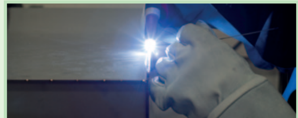
Outstanding weldability is among the assets of austenitic stainless steels like grade 304.
