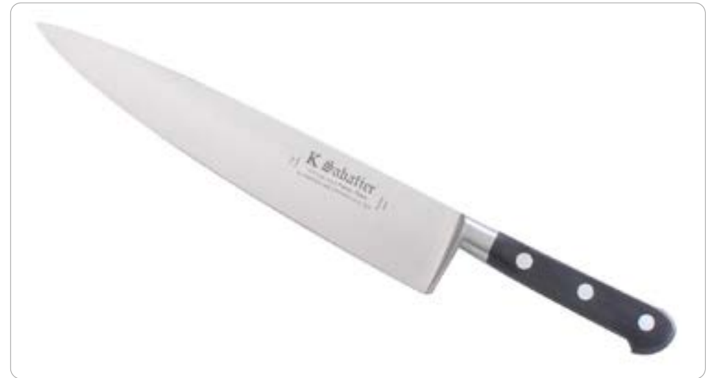
Professional carving knife, made of martensitic stainless steel grade with 0.5%C and 13%Cr forged and heat treated to a hardness of 55HRc. Courtesy of Sabatier-K.
