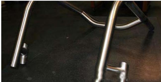
High strength stainless steels such as work-hardened austenitic or duplex stainless steel grades can be instrumental in reducing materials thickness and hence weight in structural components of wheelchairs. Photo: KVA Stainless, Escondido, CA, USA
