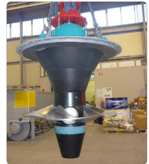
Kaplan micro hydro turbines Right: Standard Kaplan in Cannunciato, Italy Power: 870kW Head: 11m Flow: 9m 3 /s Picture courtesy of Gugler GmbH, Austria Top: Spiral Kaplan in Lapradelle Puilaurens, France Power: 98kW Head: 11.7m Flow: 0.98m 3 /s Picture courtesy of Hydrohrom s.r.o. Czech Republik
