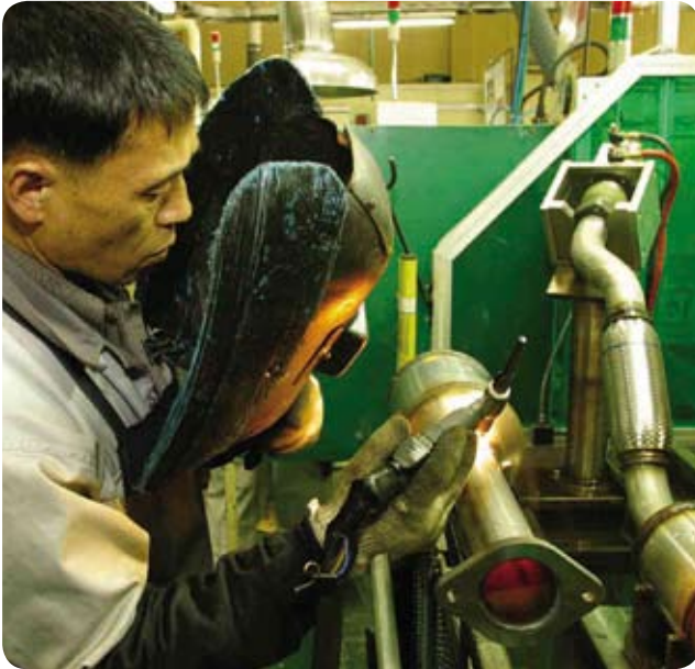
Exhaust system welding, grade 439, S. Korea.
