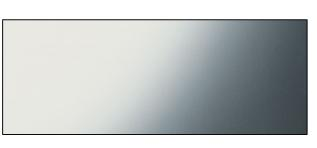
2R By bright annealing under Oxygen-free atmosphetic conditions following cold rolling using polished rolls, a highly reflective finish, that will reflect clear images, is obtained. This ultra-smooth surface is less likely to harbour airborne contaminants or moisture than any other mill finish, and it is easy to clean.
