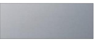
2D This is achieved by cold rolling, heat treating and pickling. The low reflective matt surface appearance is suitable for industrial and engineering needs but, architecturally, is suitable for less critical aesthetic applications.
