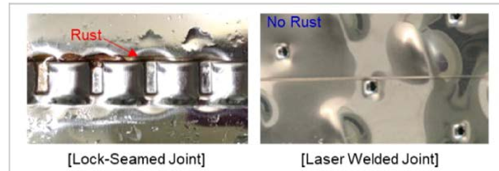
| The appearance of joint in Drum Center after corrosion test
