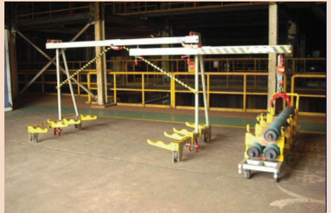
The new roll-change equipment
