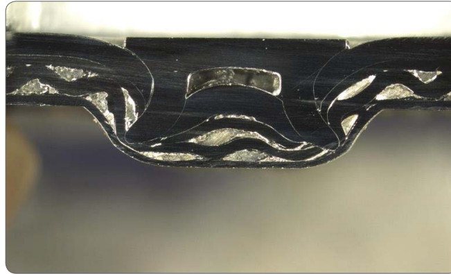
Outokumpu´s Stainless Weldable Sandwich offers also a high ability to other joining methods like the mechanical joining process of riveting. Because of the stainless 3D profiled core, the connection results in an outstanding power transmission with an enormous, state of the art not possible compressive rigidity. Background is the possibility to work out an interlocking between the profiled core inside the sandwich and the rivet.
