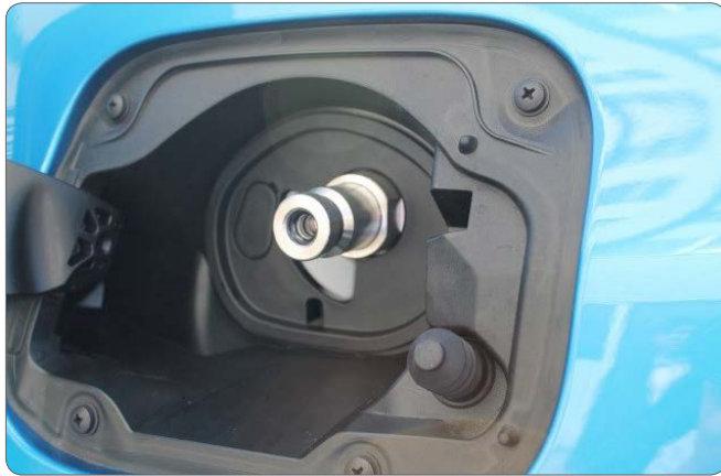
MIRAI's Hydrogen Fueling Receptacle.
