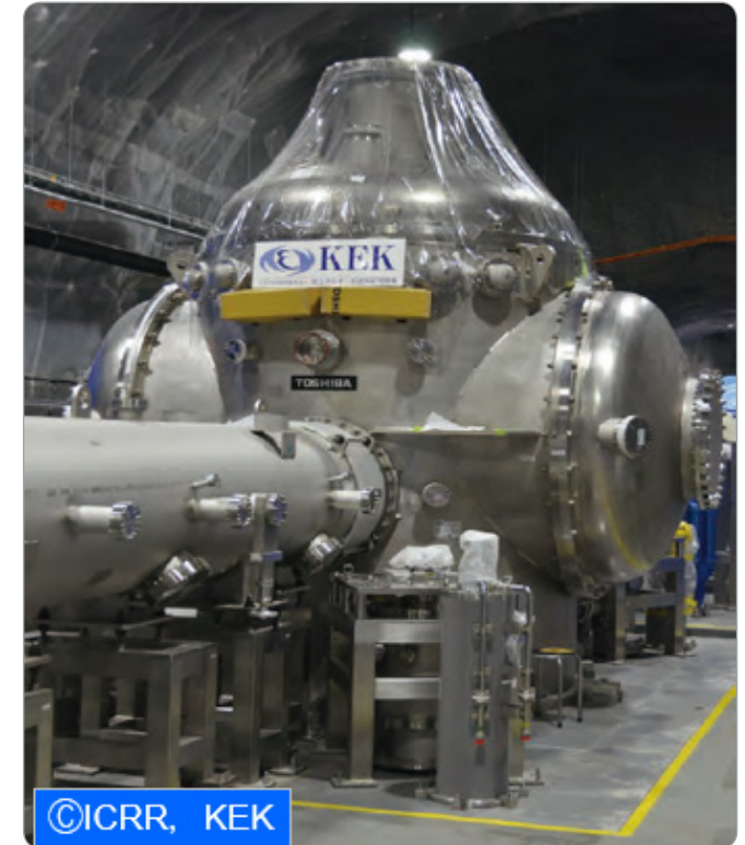
Photo 3: Cryostat (as a container for high purity crystal sapphire mirror, and so on)
