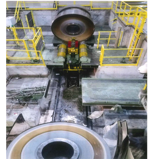
NAS Picture 3: in this picture you can see that the coil has slid off onto the floor and shot the coil car back into the coils on the saddles causing damage to these coils as well
