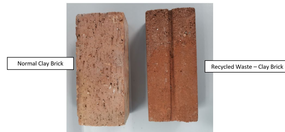
Bahru Stainless picture 1: Recycled Clay Brick versus Common Clay Brick
