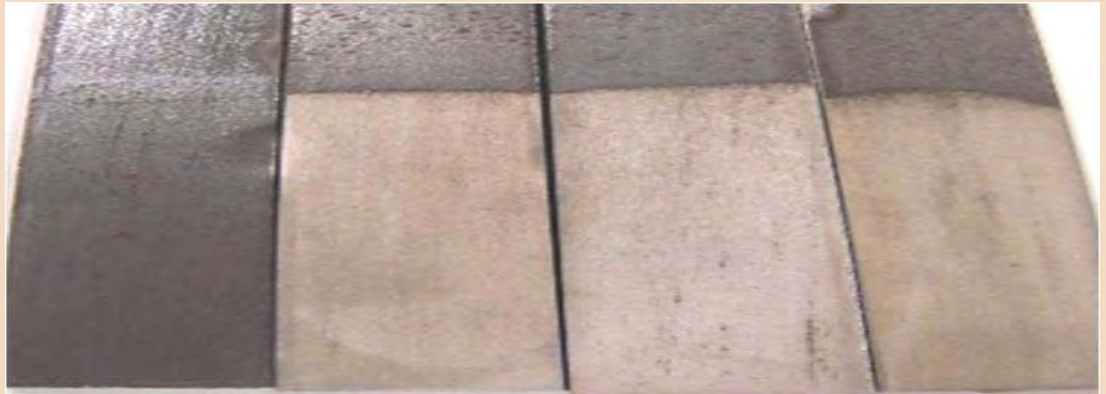
Tests were done on grade ASTM S44500 using progressively higher concentrations of H_2SO_4 (highest concentration on right)
