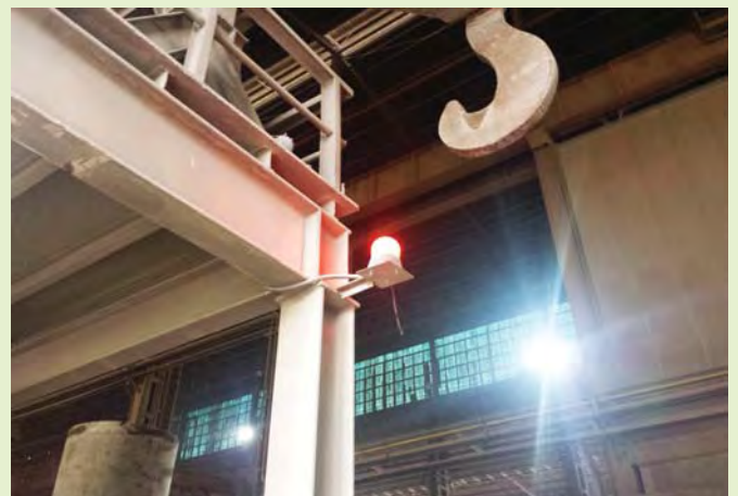
Warning lights around the plant alert workers that the crane is moving
