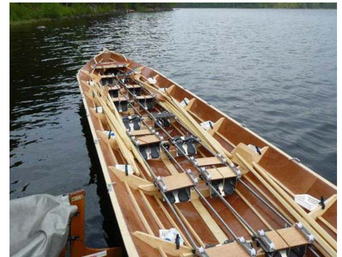
Sliding seat system with grooved rollers sliding on round stainless steel guide rails. Rugged, comfortable and low maintenance design.
