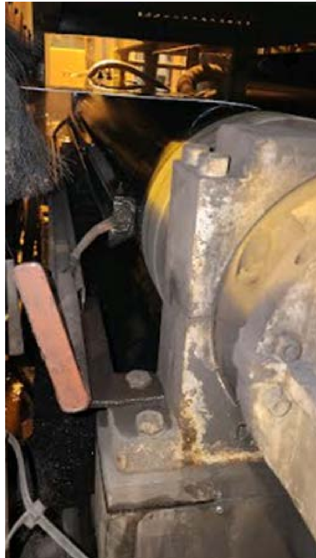
Image 2: New polisher pressing against roll while line is in operation. From the picture one can see the space is very restricted and that it would be very difficult form someone to clean the roll.
