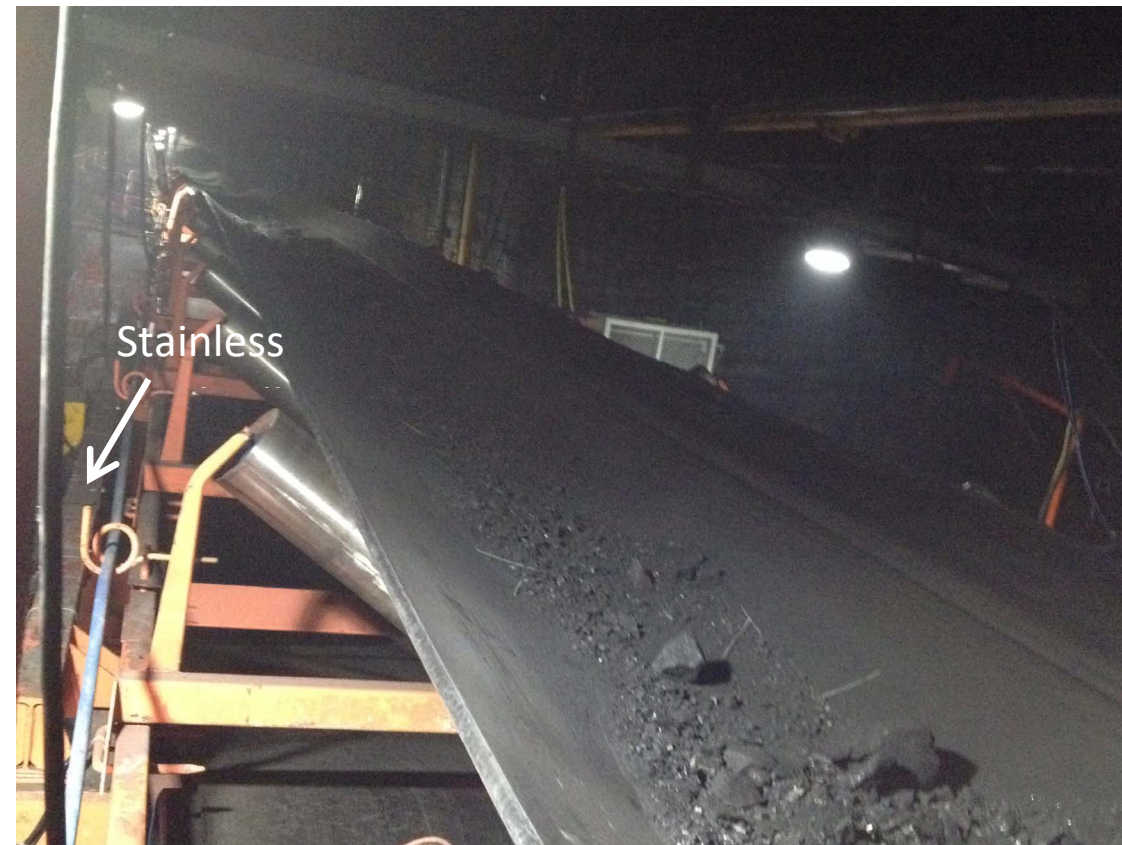
Figure 3: Stainless steel rollers in service with a bright surface
