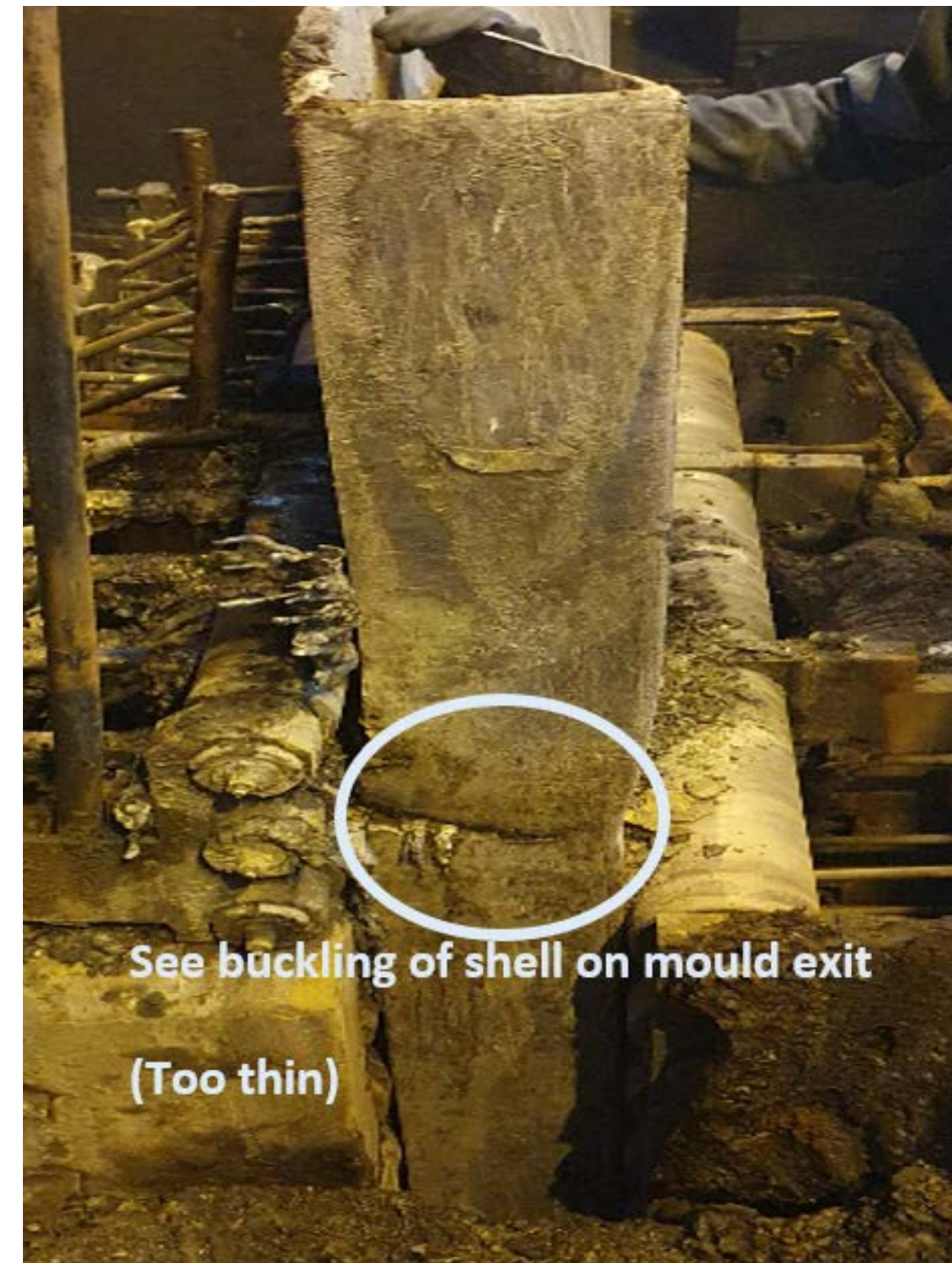
Figure 5. Thin Shell Breakout
