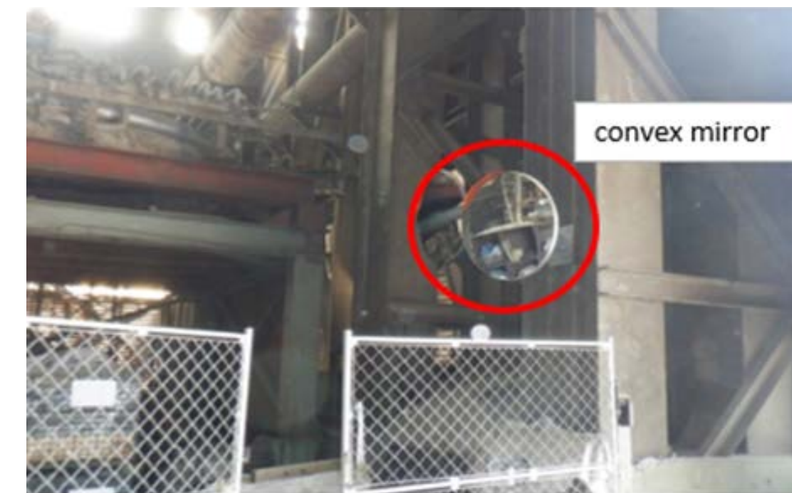
The example of the convex mirror installed in the gas blowing station of CC.
