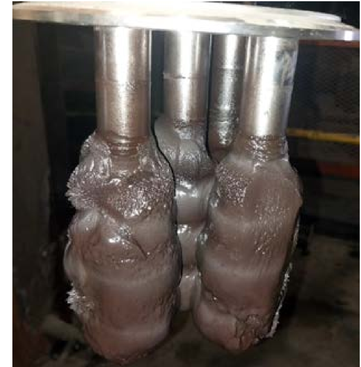
Figure 5. Magnetic debris removed on magnetic poles.
