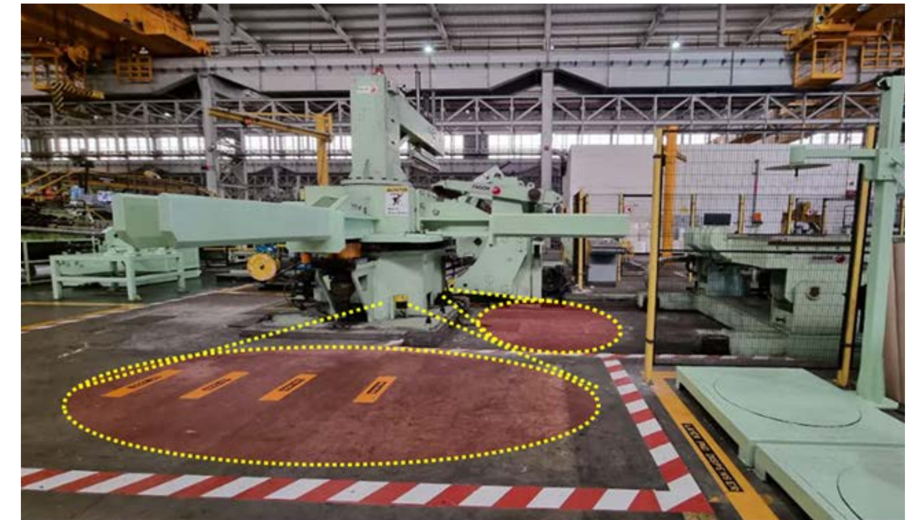
The picture indicates the smart safety zone coverage after the implementation at the machine.
