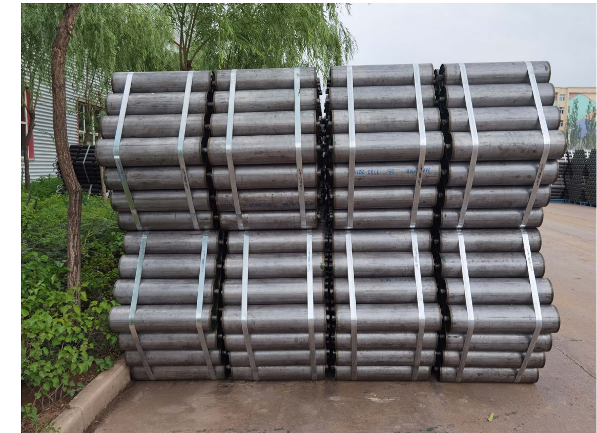
Figure 2: Stainless steel rollers for coal belt conveyor (Newly developed stainless steel)
