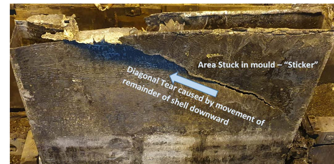
Figure 2. Sticker breakout showing the clear diagonal tear propagating towards the top of the strand.
