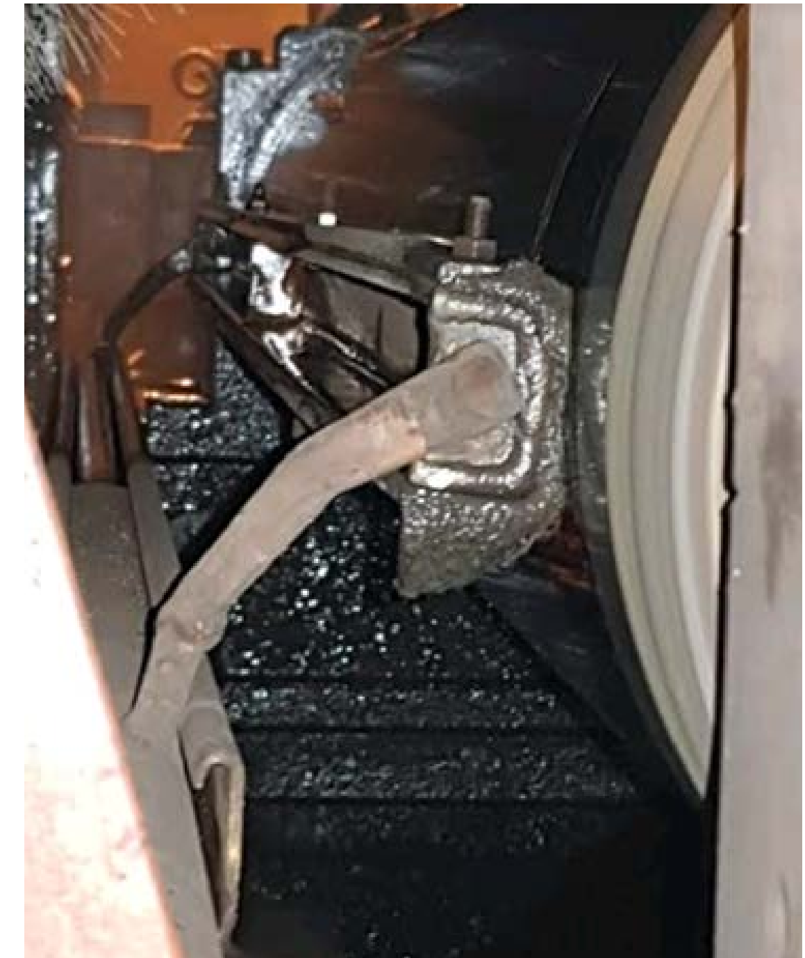
Image 3: Enlarged picture of the new polisher cleaning the roll on its own.
